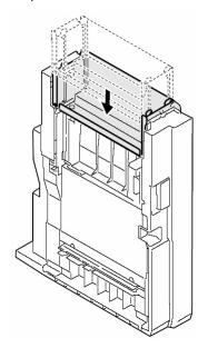
6. Reattach the extension plate using the screws you removed earlier.
